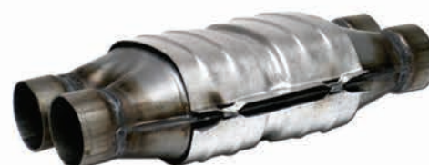
CAT907M Inlet Pipe Diameter= 50mm Outlet Pipe Diameter= 50mm Body Dimensions= 180x115mm Body Length without ending tubes= 300mm Metallic Substrate Euro3 / 200cps For engines up to 4.0 L Suitable for BMW & MERCEDES
