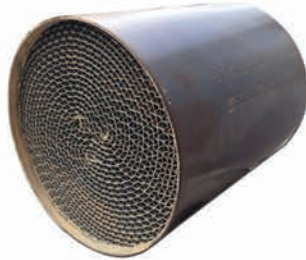
90603204 Diameter= 108mm Length= 100mm 100cpsi(Cells) PE (Perforated Foil to reduce weight & Backpressure)
