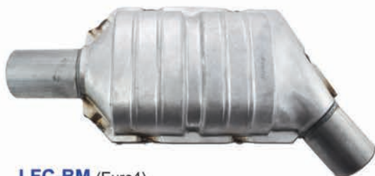
LFC-BM (Euro4) Inlet Pipe Diameter= 60mm Body Dimensions= 180x100mm Body Length without ending tubes= 330mm Metallic Substrate 400cps / High Loading For engines up to 3.0 L Suitable for BMW & MERCEDES
