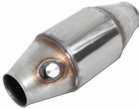
CAT110R2 Inlet=63.5mm, Body Diameter=114mm Total Length=300mm Metallic substrate 200cpsi / Euro4 Designed for performance road vehicles
