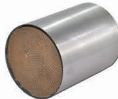
SUB52 Diameter= 120mm Length= 130mm Euro5 / 200cpsi(Cells) High Loading / Premium Quality
