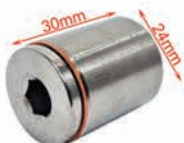
501061 S/Steel 304 Lambda boss+Plug M18 Φ24 L=30
