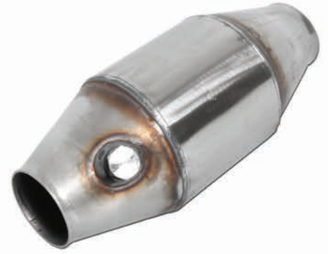
CAT125R2 Inlet=63.5mm, Body Diameter=127mm CAT125R2-3 Inlet=76mm, Body Diameter=127mm Total Length=300mm Metallic substrate 200cpsi / Euro4 Designed for performance road vehicles
